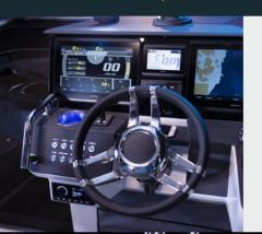
The clean driver-focused helm is designed ergonomically; all panels and switches are centrally positioned around the skipper. The console fits two 12" Garmin plotters.
